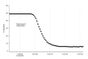
This diagram shows a typical pattern of a phase change from Juice to water, which takes place within about 20 seconds. The PhaseGuard C picks up this interface change quickly and with high precision. It allows the user to select the switching point which he believes is the optimum (compromise between juice loss or amount of water for the rinsing). Up to now timers have been used and times often set to ensure an over-rinse condition.
