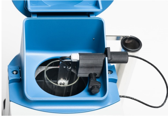
Pict. 5: LabScat with inserted cuvette & temperature sensor (lid open)
